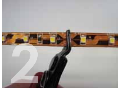
2 CUT BETWEEN SOLDER CIRCLES ON THE DESIGNATED LINE AS SEEN IN STEP 1.
