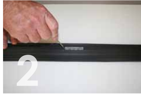
TO REPLACE LED CIRCUIT BOARD, FIRST TURN OFF THE POWER. THEN SLIDE A SMALL SCREW DRIVER DOWN BETWEEN THE LEDTread EXTRUSION AND LENS CAP. CAREFULLY BEGIN TO PRY THE LENS CAP UP.
