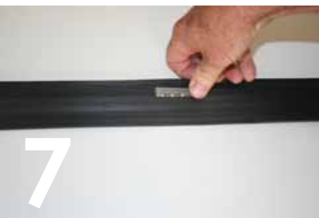
PLACE NEW LED CIRCUIT BOARD BACK ONTO THE TWO BRASS PINS MAKING SURE NOT TO BEND THE PINS. PUSH DOWN TO INSURE A GOOD CONNECTION.
