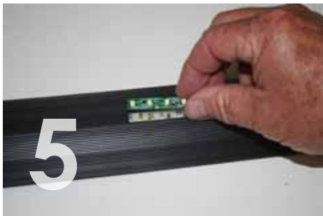
PLACE NEW LED CIRCUIT BOARD BACK ONTO THE TWO BRASS PINS MAKING SURE NOT TO BEND THE PINS. PUSH DOWN TO INSURE A GOOD CONNECTION.
