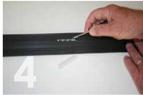
CAREFULLY SLIDE SCREW DRIVER UNDER THE EDGE OF THE LED CIRCUIT BOARD AND REMOVE THE BOARD OFF THE TWO BRASS PINS IN THE MODULE.
