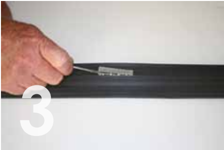
AFTER BOTH LENS CAP LEGS ARE RELEASED FROM THE MODULE REMOVE THE LENS CAP.
